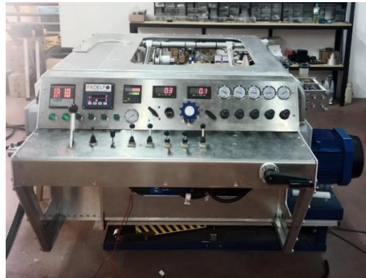
Figure 5: Pressure Control Panel (left) and Operations Winch (right).
