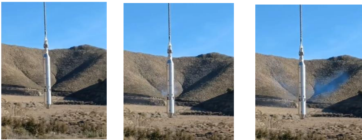
Figure 2: Illustration of the sequence for generating the discharge of compressed air at 150 bars using the pulse generator.
